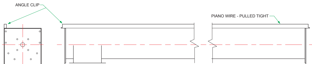
CEMA COMMONLY USED PIANO WIRE SETUP Piano wire attached to top of conveyor on side
